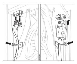
■ Plug the 2 connectors on the canopy into the corresponding receptacles left and right of the motor assembly.
